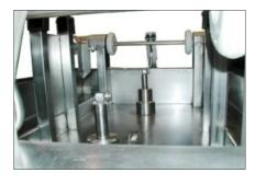
The AaquaBlaster LT AUTOMATIC features an automatic barrel positioning system.
