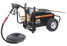
The Mi-T-M Portable Pressure Washer is just the workhorse you need to power our Tilt Truck Washer. The belt driven triplex piston pump is a powerhouse that delivers 12 gpm at 1500 psi and
